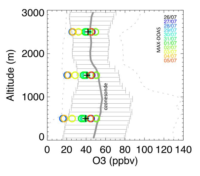
MAX-DOAS  $O_3$  partial column (<1 km, circles) observations simulated with a box model (van Stratum et al., 2012). Simulations (lines) used the ABLH, [NO2] and [HCHO] observed at 10 am as initial conditions. In these days, clean maritime air masses bring very low O3.
